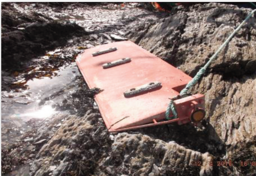
Photograph No. 3: Rudder lying on rocks beside vessel.
