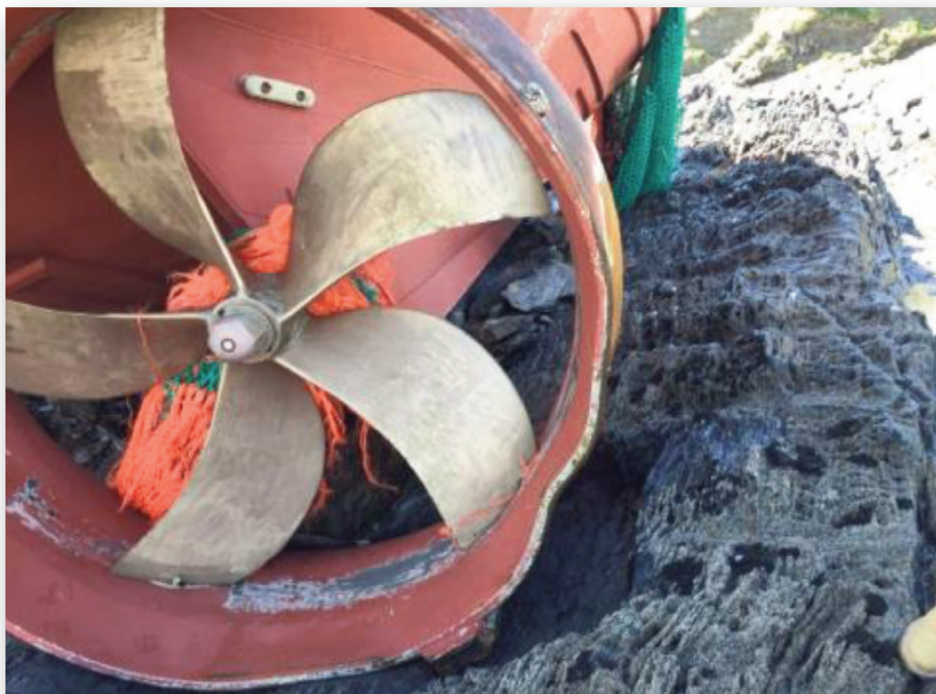
Photograph No. 1: Rope wrapped around inboard part of propeller.
